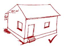
For sloping roof, the slope should be between 22 degrees to 30 degrees. Roof overhang must be no more than 500mm (20") in rainy areas.
