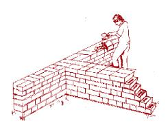
Build all the walls together at each course Or else, leave the end of the wall in a stepped/zig-zag manner for connecting later.
