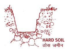
Decide the depth of foundation depending on how strong the ground is. Soft soils require deeper foundation than hard soil.
