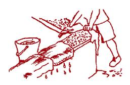
RCC beams and columns must be kept wet using jute bags / hessian for 10 days.
