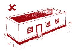
even collapse easily than a shorter building. Avoid constructing a house with length more than 2 times its width. Otherwise divide the building in two separate units. बहुत अधिक लंबे भवन आसानी से क्षतिग्रस्त हो
