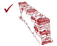
When building with stones, place through stones into the thickness of wall to ensure interlocking of inside and outside faces of the wall.
