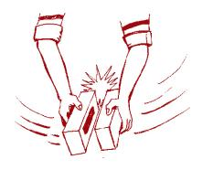
A metallic sound is produced when two good quality bricks are struck.
